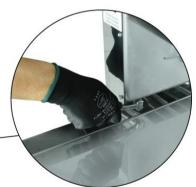
After fixing the table, place the machine on a stand with an average height of 80 cm in a sufficiently wide, level, dry and stable area, away from heat sources, water faucets and areas with high circulation of people. Install the machine leaving a free area on the front and a minimum distance of 50 cm on the sides and back so there is enough space for inspection, maintenance, cleaning and use.
