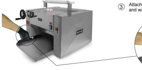
3 Attach the table using the four screws and washers using an appropriate tool.
