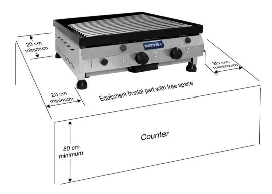
It is recommended to install a hood or extractor above the equipment to collect vapors, preventing them from spreading into the environment.
