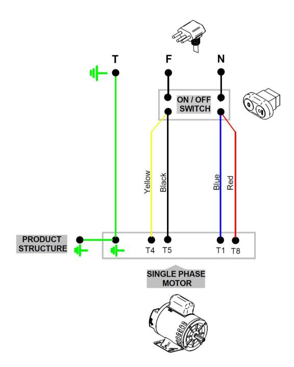
NOTE: Motor with dual direction of rotation. To reverse rotation, change T5 to T8.
